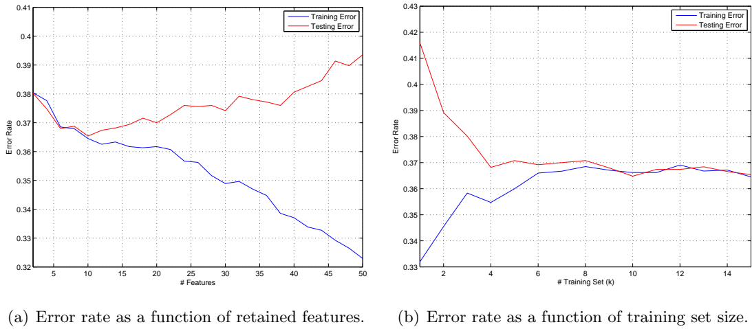
Figure 5.16: Error rate for CIOS Montgomery multiplication architecture traces.
